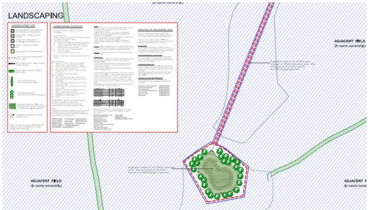
Proposed Part Site Layout Plan – Drawing Extract GO6 with landscaping and swale drainage
