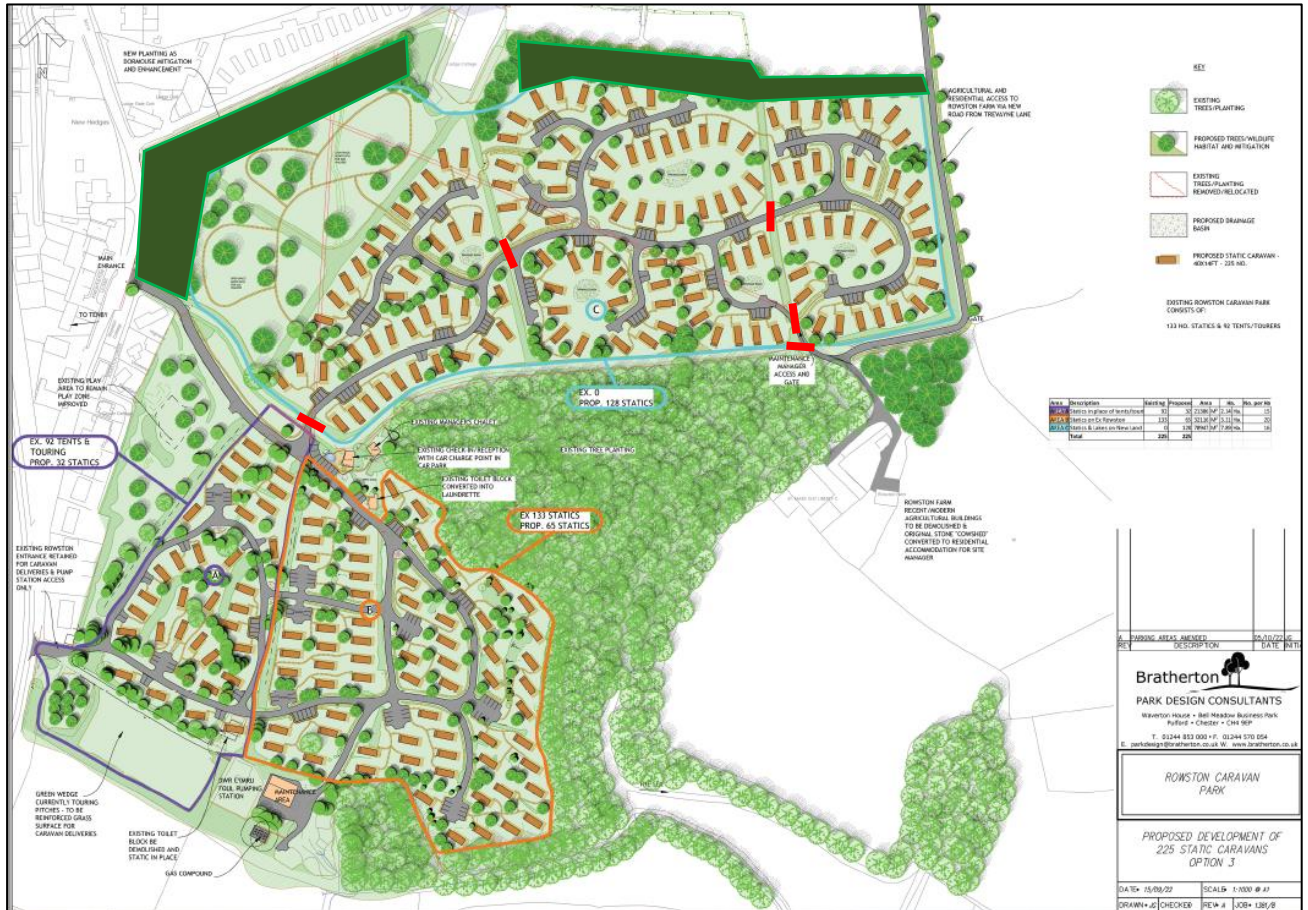
Figure 32. New access points (in red) in relation to proposed new planting (green).
