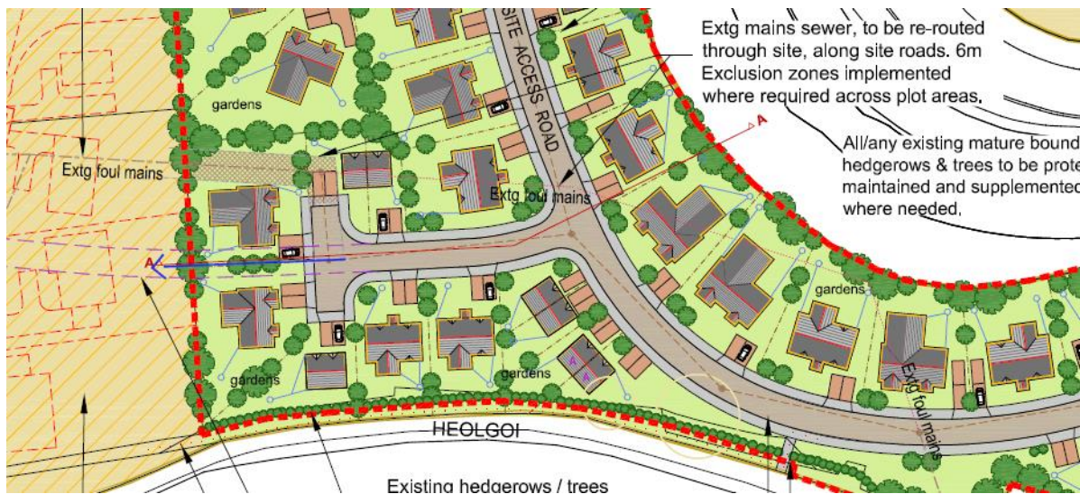
Extract of drawing P02, Site Layout, showing the proposed diversion of the foul mains sewer
